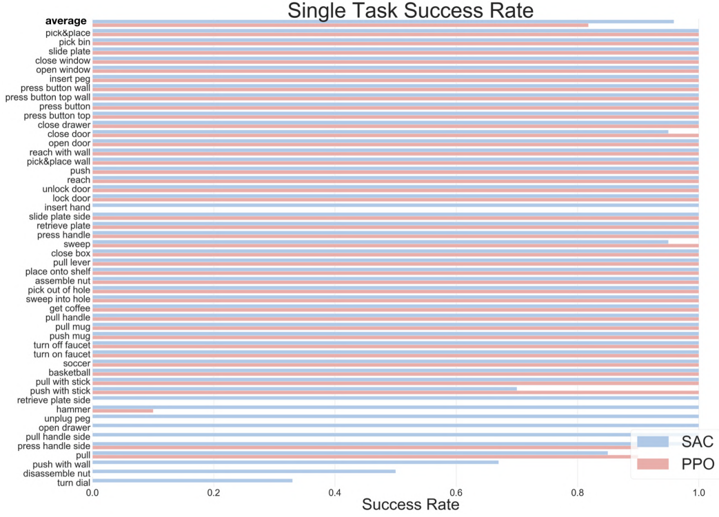
Figure 6: Performance of independent policies trained on individual tasks using soft actor-critic (SAC) and proximal policy optimization (PPO). We verify that SAC can solve all of the tasks and PPO can also solve most of the tasks.
