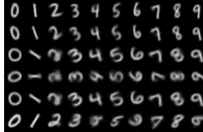
Figure 5: Visualizing VAE samples conditioned on different values of y (x axis) and c (y axis). The VAE learns to use c to represent rotations.
